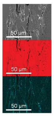
Fig. 8 The cross-section of sheets containing 10% of nanoparticlelabeled materials. The elemental distribution was evaluated by energy dispersive X-rays, thereby revealing a uniform distribution of carbon (red), while the distribution of cobalt (cyan) has the form of fibrils. The image is reprinted from Hobisch et al. 172 Copyright (2021), with permission from Elsevier.
