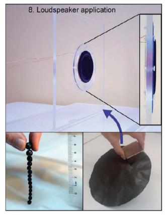
Fig. 6 A magnetic membrane (bottom right) prepared by vacuum filtration of magnetic nanofibril suspension in a thin prototype loudspeaker operating without an external magnet (upper figure). Hard permanently magnetized spherical beads are shown in bottom left figure. The image has been reproduced from Galland et al. 114 under CC BY-NC 3.0 license.
