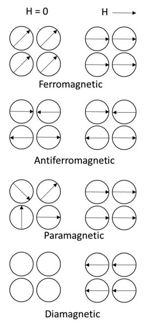
Fig. 3 Illustration of the magnetic dipole moments in magnetic materials with and without an external magnetic field (H).
