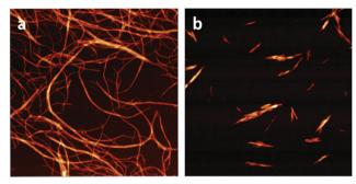
Fig. 2 Atomic force microscopy visualization of cellulose nanofibers (a) and cellulose nanocrystals (b). The frame size is 3  $\times$  3  $\mu m$ .
