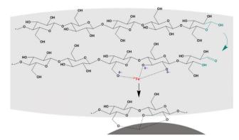
A scenario of coordination of a metal ion (red) with cellulose molecule or hierarchy (presented by light grey area) that. The nucleation into particles (dark grey), via co-precipitation, leads to cellulose hybrids. Reducing end group (green, the arrow indicates the two available forms, the open form and hemiacetal form) is available for modification. The asterisk (\*) indicates the fact that the cellulose chain continues
