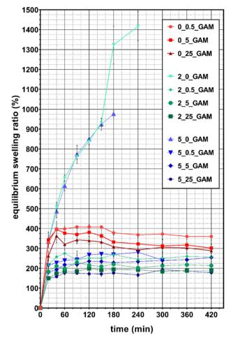
Fig. 5 Equilibrium swelling ratio of lyophilized GAMs depending on the cross-linking method and the concentrations of cross-linking agents. A chart uses points connected by line segments from left to right to demonstrate changes in value and to facilitate tracking of them.
