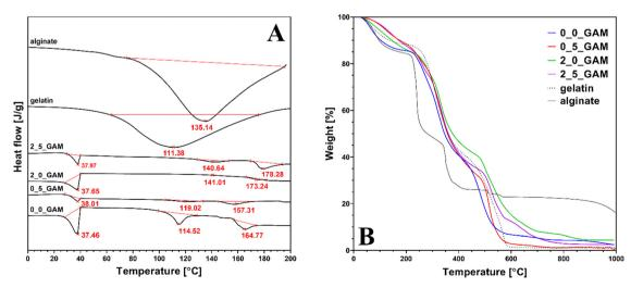
Fig. 4 (A) Differential scanning calorimetry and (B) thermogravimetric analysis of pure gelatin, sodium alginate and GAMs results.
