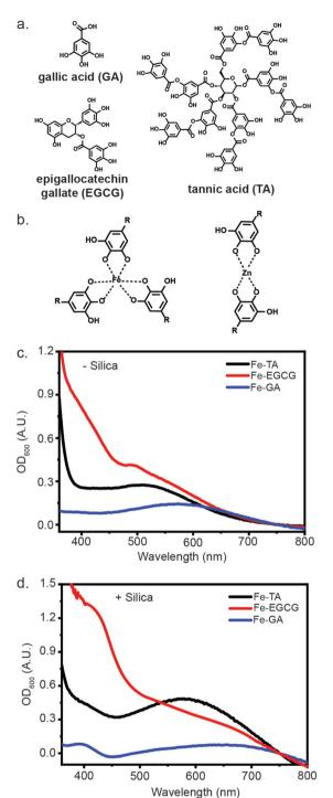
Fig. 1 Abiotic characterization of metal-phenolic networks (MPNs). (a) Polyphenol components used in the MPN assemblies. (b) Example chelation of metal ions (Fe $^{\rm III}$  and Zn $^{\rm II}$ ) to polyphenols. (c) UV-Vis absorbance of Fe $^{\rm III}$ -TA, Fe $^{\rm III}$ -GA, and Fe $^{\rm III}$ -EGCG complexes in MOPS buffer (10 mM, pH 7.5). (d) Fe $^{\rm III}$ -TA, Fe $^{\rm III}$ -GA, and Fe $^{\rm III}$ -EGCG complexes formed on the surface of silica particles (1 mg mL $^{-1}$ ).
