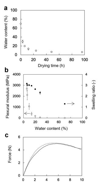
Fig. 4 (a) Water contents (WC) of rectangular PVA hydrogels as a function of drying time. (b) Flexural moduli and swelling ratios of rectangular PVA hydrogels as a function of WC. Data are presented as the mean  $\pm$  SD (n =3). (c) Force-deformation curves of the tube-shaped PVA hydrogel (solid line) and PS (dotted line).
