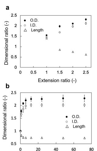
Fig. 1 Changes in the dimensional ratios of the outer diameter (O.D.), inner diameter (I.D.), and length of tube-shaped PVA hydrogels as a function of (a) the extension ratio and (b) the immersion time in physiological saline for a hydrogel with an extension ratio of 2.0. Data are presented as the mean  $\pm$  SD (n = 3)
