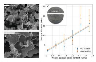
Fig. 3 Physical properties of GO foam and rGO foam scaffold. (a) and (b) SEM images showing the typical porous structure of the dry 2.00 wt% foam. (c) Scaffold Young's modulus increases linearly with solid contents in the foam, demonstrating control over scaffold properties. Inset is an optical photograph of a whole foam scaffold sample showing cylindrical mould geometry.
