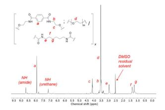
Fig. 2  $^{1}$ H NMR of the 1BHETA:2PEG polyurethane in d<sub>6</sub>-DMSO.
