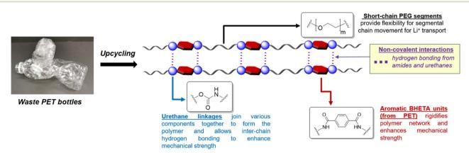
Fig. 1 Design of polyurethane polymer electrolytes derived from waste PET with hard (aromatic) and soft (PEG) components.
