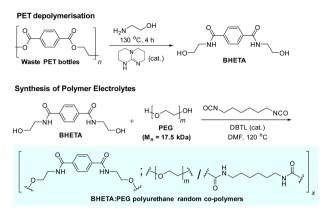
Scheme 1 Synthesis of BHETA:PEG polymer electrolytes from waste
