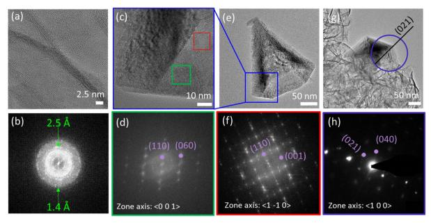
Fig. 6 (a and b) HRTEM micrograph and corresponding FFT pattern of a HMO nanosheet. (c-f) HRTEM micrographs and FFT patterns corresponding to two facets of a FMO2 nanocone. (q and h) TEM micrograph and corresponding SAED pattern of a FMO2 nanocone.
