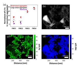
Fig. 3 (a) Normalized at% Fe with respect to at% Mn for each material. (b-d) HAADF micrograph and corresponding EDS mapping after PCA analysis showing the distribution of Fe and Mn on nanosheets and nanocones in FM02.
