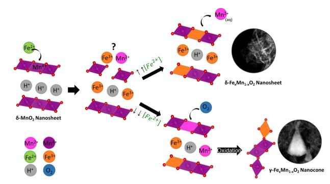
Fig. 7 Schematic mechanism governing the synthesis of  $Fe_vMn_{1-v}O_2$  nanosheets and nanocones through galvanic exchange reaction.
