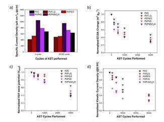
Fig. 3 ORR parameters across the 1–1.6  $V_{RHE}$  AST for different functionalised FLG materials and Pt/C over 30 000 corrosion cycles. (a) Specific current density (at 0.9 V) for each material at 0 and 30 000 cycles. (b) Normalised ECSA change across the 30 000 of AST. (c) Normalised half wave potential change across the 30 000 of AST. (d) Normalised kinetic current density (at 0.9 V) change across the 30 000 of AST
