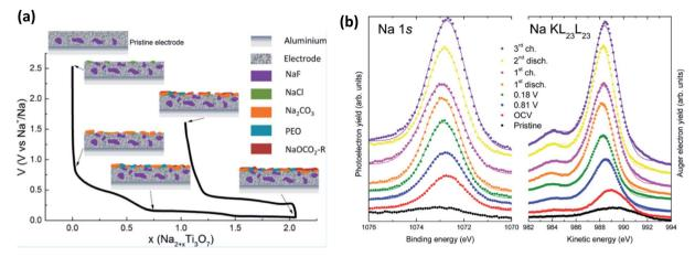
Fig. 13 (a) The composition and evolution of the SEI on Na<sub>2</sub>Ti<sub>2</sub>O<sub>7</sub> electrodes as determined by XPS. (b) Na 1s XPS spectra and Na KL<sub>23</sub>L<sub>23</sub> Auger transition spectra for electrodes at different states of charge. Reprinted with permission from ref. 143. Copyright 2015 American Chemical Society
