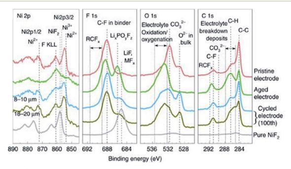
Fig. 10 XPS spectra (Ni 2p, F 1s, O 1s, C 1s) of LiNi $_{0.7}$ Mn $_{0.15}$ Co $_{0.15}$ O $_2$  electrodes (pristine, aged, and cycled electrodes with 8–10 and 18–20  $\mu$ m particle sizes) and pure NiF $_2$ . Reproduced under CC-BY licence from ref. 107.
