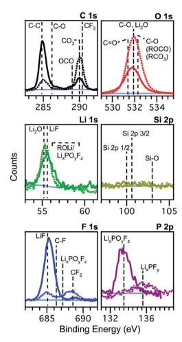
Fig. 4 XPS spectra of silicon (001) wafer electrodes after preparation by chronoamperometry at 0.01 V vs. Li<sup>+</sup>/Li for 300 s in an electrolyte of 1 M LiPF<sub>6</sub> in ethylene carbonate (EC) and diethyl carbonate (DEC), 1:1 w/w. Solid lines: measured without exposure; dashed lines: measured after exposure to the atmosphere for 10 minutes. Reprinted with permission from ref. 56. Copyright 2012 American Chemical Society.
