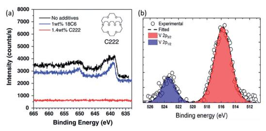
Fig. 12 (a) Mn 2p spectra of graphite electrodes after 5 cycles with  $LiMn_2O_4$  cathodes in 1 M  $LiClO_4/EC + DEC$  with and without the 18C6 or C222 cyclic ether additives. Reproduced from ref. 119 with permission from the Royal Society of Chemistry. (b) V 2p core level of the vanadium deposited on the anode. Reprinted with permission from ref. 122. Copyright 2019 American Chemical Society.
