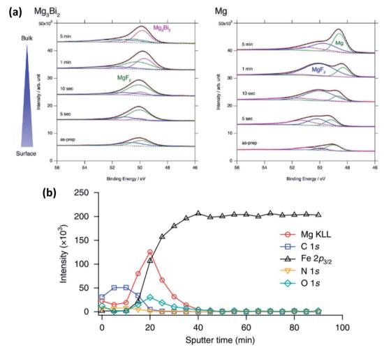
Fig. 18 (a) Mg 2p XPS spectra after sputter-etch depth profiling for  $Mg_3Bi_2$  and Mg thin films immersed in 0.5 mol  $L^{-1}$  Mg(TFSA)<sub>2</sub> in BuMeG3 solution for 24 h. Reproduced under CC-BY licence from ref. 155. (b) XPS sputter-etch depth profiles of a Mg-coated stainless-steel electrode in 0.5 M Mg(TFSI)<sub>2</sub>-PC electrolyte. Reprinted by permission from Nature Chemistry<sup>156</sup> Copyright 2018.
