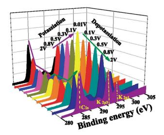
Fig. 17 K 2p-C 1s XPS spectra of hard carbon electrodes at various states of charge from potassium systems, showing the increase and subsequent decrease in the substrate signal. Reprinted from ref. 150, with permission from Elsevier.
