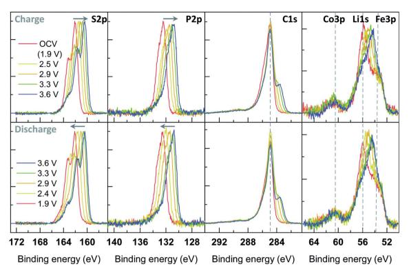
Fig. 29 Operando XPS experimental results during potentiostatic measurement of a working electrode made of 45 wt% LCO, 50 wt% amorphous (Li<sub>2</sub>S)<sub>3</sub>-P<sub>2</sub>S<sub>5</sub> and 5 wt% VGCF cycled vs. InLi<sub>x</sub>. Reprinted from ref. 182
