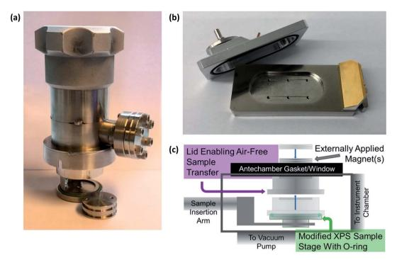
Fig. 5 Devices for air-sensitive transfer of samples to XPS instruments. (a) Sample transfer cup for PHI 5500 XPS instrument. (b) Air-sensitive sample shuttle for Kratos AXIS Supra+. (c) A magnetic sealing sample holder: Reprinted with permission from ref. 60. Copyright 2020 American Chemical Society.
