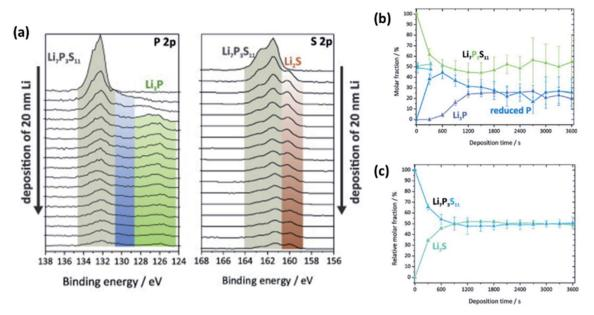
Fig. 26 (a) In situ XPS measurements of  $\text{Li}_7P_3S_{11}$  solid electrolyte on which Li is deposited. Relative molar fractions of (b) phosphorus and (c) sulphur species for different times of Li deposition. Reprinted from ref. 192, with permission from Elsevier.
