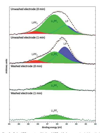
Fig. 6 F 1s XPS spectra (Al Kα, 1487 eV) from washed (dimethyl carbonate (DMC), 2 min, dried in argon) and unwashed graphite anode from full cells with LiCoO2 cathode and electrolyte of 1 M LiPF6 in ethylene carbonate (EC)/ethyl methyl carbonate (EMC), 3:7 w/w. The minutes in the figure refer to the duration of Ar<sup>+</sup> sputtering before XPS measurement. Reproduced under CC-BY licence from ref. 66.
