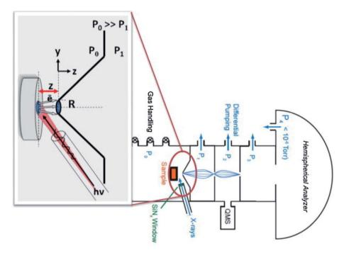
A schematic illustration of an APXPS instrument. Reprinted from ref. 211, with permission from Elsevier.
