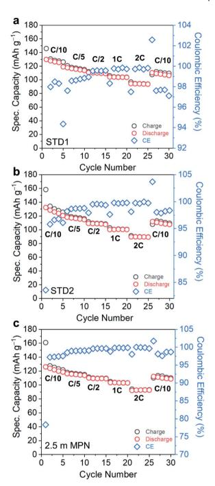
Fig. 4 Rate capability performance of  $gr\|LCO$  cells when subjected to C-rates ranging from C/10 to 2C and utilizing (a) STD1, (b) STD2, and (c) 2.5 m MPN electrolytes.
