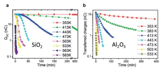
Fig. 8 Charge dissipation by thermionic emission. Amounts of static charge on (a)  $SiO_2$  and (b)  $Al_2O_3$  surfaces as a function of time under different temperatures. Reproduced with permission (copyright 2018, Wiley-VCH).<sup>122</sup>
