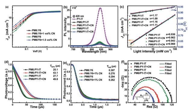
Fig. 3 (a)  $J_{ph}-V_{eff}$  curves of all-PSCs. (b) Photoluminescence spectra of the PY-IT film, and PM6:PY-IT and PM6/PY-IT blend films under 420 nm light excitation. (c)  $J_{\rm sc}-P_{\rm light}$  and  $V_{\rm oc}-P_{\rm light}$  curves of all-PSCs. (d) Transient photovoltage curves of all-PSCs. (e) Transient photocurrent curves of all-PSCs. (f) Nyquist plots and the equivalent circuit of all-PSCs.
