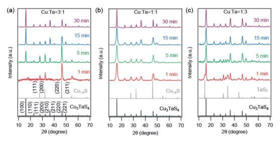
Fig. 2 XRD patterns of synthesized Cu-Ta-S NCs for (a) Cu: Ta = 3:1, (b) Cu: Ta = 1:1, and (c) Cu: Ta = 1:3 reactions, collected at different reaction times. The standard cubic phase of  $Cu_3TaS_4$  ( $P\bar{4}3m$ ) and  $Cu_{2-x}S$  ( $Fm\bar{3}m$ ; x=0.2) are shown by black and grey solid line.
