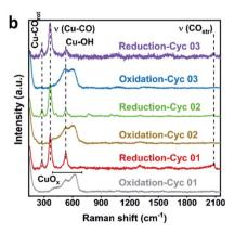
Fig. 4 In situ Raman studies on oxidized Cu species of Cu/PTFE. (a) In situ SERS of Cu/PTFE conducted at different times of reaction in  $KHCO_3$  electrolyte at a current density of 30 mA cm<sup>-2</sup>. (b) The structure and surface adsorbates during reduction and oxidation cycles at 0.6 mA cm<sup>-2</sup> oxidation current density for 20 s.
