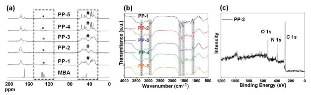
Molecular characterization of porous polymers via (a) solid state <sup>13</sup>C NMR spectra, (b) IR spectra and (c) XPS spectra.
