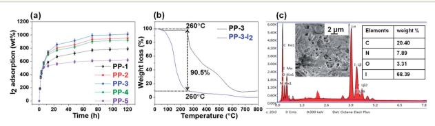
Fig. 4 (a) Iodine adsorption of PPs in the vapor phase, (b) TGA analysis and (c) SEM and EDX analyses of iodine adsorbed porous polymers.
