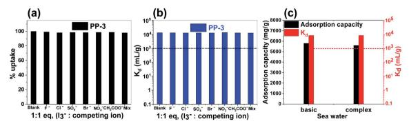
Fig. 7 (a) Uptake percent for  $I_3^-$  anions in the presence of other competing anions, (b) distribution coefficient ( $K_d$ ) graph and (c)  $I_3^-$  adsorption capacity from the basic and complex seawater and the corresponding distribution coefficient value  $(K_d)$ .
