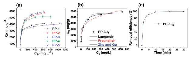
Fig. 6 lodine adsorption study in water: (a) adsorption isotherms of different porous polymers, (b) Langmuir, Freundlich and Zhu and Gu adsorption isotherm models for PP-3, and (c) iodine adsorption kinetics.
