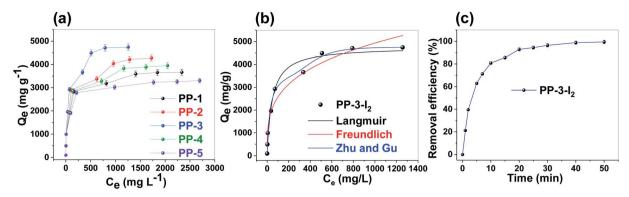
Fig. 5 lodine adsorption study in n-hexane: (a) adsorption isotherms of different porous polymers, (b) Langmuir, Freundlich and Zhu and Gu adsorption isotherm models for PP-3, and (c) iodine adsorption kinetics.
