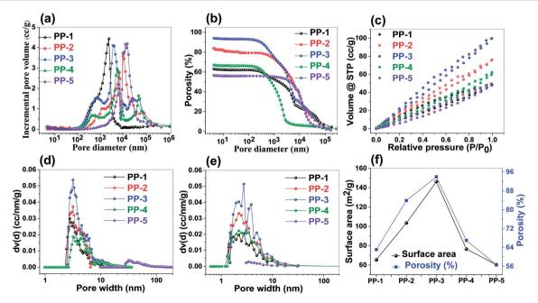
Fig. 2 Porosity and surface area analysis of the porous polymers (a) pore size distribution by mercury porosimetry, (b) calculated overall porosity, (c) nitrogen adsorption desorption isotherms at 77 K, pore size distribution of the PP as determined by (d) DFT and (e) the BJH method and (f) comparison graph between the porosity and surface area of all porous polymers.
