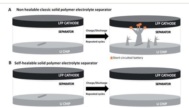
Fig. 1 (A) Scratched classic SPE separator before and after repeated charge and discharge cycles. (B) Scratched self-healable SPE separator to avoid dendrite growth after repeated charge/discharge cycles.
