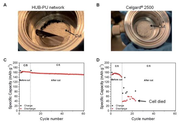
Fig. 5 (A and B) Optical proof of the cut carried out inside the glove box on both the self-healable HUB-PU network and Celgard® 2500 membrane after 10 cycles at C/5 rate. (C and D) Specific capacity (mA h g<sup>-1</sup>) vs. cycle number at C/5 rate for the HUB-PU network and Celgard® 2500 membrane, respectively. The first 10 cycles are carried out before the cut, while the subsequent cycles refer to the period after the cut.
