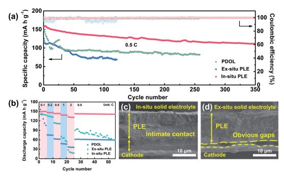
Fig. 5 (a) The long-term cycling stability of Li|LFP full batteries at 0.5C. (b) The rate capability of full batteries with different electrolytes. Cross-sectional views of the cycled Li|LiFePO<sub>4</sub> batteries assembled with (c) In-situ PLE, and (d) Ex-situ PLE.
