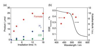
Fig. 5 (a) Time courses of photocatalytic reaction and (b) action spectra of external quantum efficiency of formate formation (EQE<sub>formate</sub>) by  $[Cz-bpyRu]_n$  (2 mg) in an MeCN-TEOA (2 mL; 4 : 1 v/v) dispersion under CO2 atmosphere
