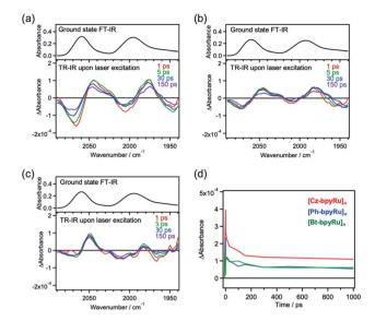
Fig. 4 Ground state FT-IR (upper) and TR-IR (lower) spectra of (a) [Cz-bpyRu]<sub>n</sub>, (b) [Ph-bpyRu]<sub>n</sub>, and (c) [Bt-bpyRu]<sub>n</sub>, along with (d) time courses of the differential absorbance at 2045 cm<sup>-1</sup> and 2069 cm<sup>-1</sup> (red: [Cz-bpyRu]<sub>n</sub>, blue: [Ph-bpyRu]<sub>n</sub>, and green: [Bt-bpyRu]<sub>n</sub>).
