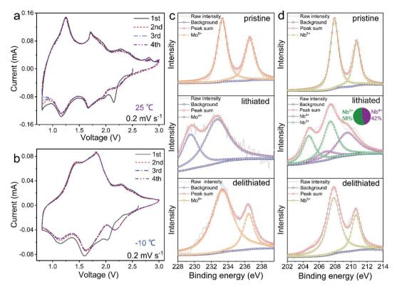
Fig. 4 Redox mechanism of Mo<sub>4</sub>Nb<sub>26</sub>O<sub>77</sub> submicron-sized particles. First four-cycle CV profiles of the Mo<sub>4</sub>Nb<sub>26</sub>O<sub>77</sub>/Li half cell at (a) 25 and (b) -10 °C. Ex situ (c) Mo-3d and (d) Nb-3d XPS spectra of pristine, lithiated and delithiated Mo<sub>4</sub>Nb<sub>26</sub>O<sub>77</sub> samples at 25 °C.
