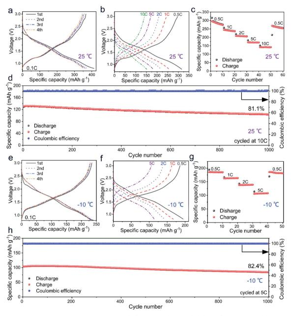
Fig. 2 Electrochemical characterization studies of the  $Mo_4Nb_26O_{77}/Li$  half cell at 25 and  $-10\,^{\circ}$ C. (a and e) First four-cycle GCD curves at 0.1C. (b and f) GCD curves at various current rates. (c and g) Rate performance. (d and h) Long-term cyclability over 1000 cycles.
