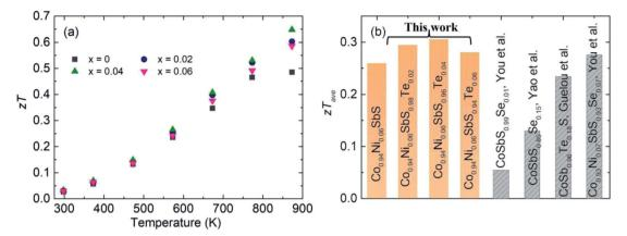
Fig. 6 zT value of the  $Co_{0.94}Ni_{0.06}SbS_{1-x}Te_x$  samples (x=0,0.02,0.04, and 0.06). (a) Temperature-dependent zT values and (b) comparison of the  $Co_{0.94}Ni_{0.06}SbS_{1-x}Te_x$  samples with other reported CoSbS samples prepared by Hou et al., Yao et al., and Guelou et al.
