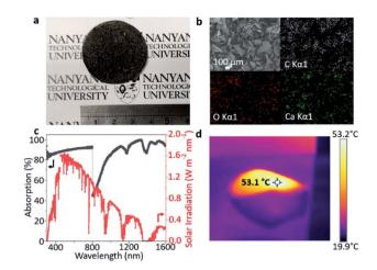
Fig. 3 (a) Photograph of 2D g-CNS<sub>PB</sub> deposited on air-laid paper, (b) FESEM image of a 2D g-CNS<sub>PB</sub> photothermal layer with its corresponding EDX mapping images of C, O and Ca elements, (c) UV-vis-NIR absorption spectrum of 2D g-CNS<sub>PB</sub> with AM 1.5 solar irradiance as a reference. (d) Thermal image of the 2D g-CNS<sub>PB</sub> photothermal layer under air.
