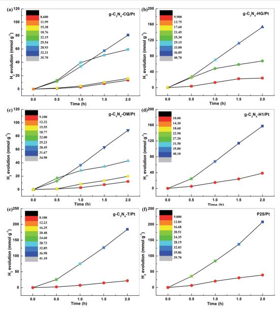
Fig. 3 The general phenomenon for STAP  $H_2$  evolution kinetics. The  $H_2$  evolution yield correlated with system temperature elevation at a variable time under simulated solar light irradiation for the photocatalyst of (a)  $g-C_3N_4-CQ/Pt$ , (b)  $g-C_3N_4-HG/Pt$ , (c)  $g-C_3N_4-DM/Pt$ , (d)  $g-C_3N_4-DM/Pt$ , (e)  $g-C_3N_4-DM/Pt$ , (f) P25 (TiO<sub>2</sub>)/Pt. Inset: color scale bar representing system temperature elevation. Photocatalyst loading, 10 mg.
