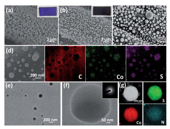
Fig. 1 SEM images of Co-MOF/CC (a) and  $CoS_x/CC-L$  (b and c). Insets are the corresponding photographs. (d) Corresponding EDS mapping of the C element, Co element and S element for  $CoS_x/CC-L$ . TEM (e) and HRTEM (f) images of  $CoS_x/CC-L$ . The inset in (f) is the SAED pattern of  $CoS_x/CC-L$ . (g) Elemental mapping of  $CoS_x$  nanospheres.
