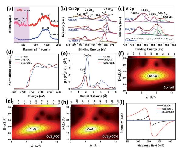
Fig. 2 (a) Raman spectra and high-resolution XPS spectra of the Co 2p (b), S 2p (c) for Co-MOF/CC,  $CoS_x/CC-L$  and  $CoS_2/CC$ . (d) Normalized Co K-edge XANES spectra and (e) Fourier transform of  $k^2$ -weighted Co EXAFS spectra of Co foil, CoS<sub>x</sub>/CC-L and CoS<sub>2</sub>/CC. (f-h) WT-EXAFS spectra of the Co foil, CoS<sub>2</sub>/CC and CoS<sub>x</sub>/CC-L. (i) EPR spectra of Co-MOF/CC, CoS<sub>x</sub>/CC-L and CoS<sub>2</sub>/CC.
