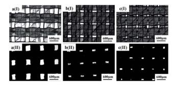
Fig. 2 Microscopic images of the prepared membranes with different pore sizes ((a),  $240 \times 400~\mu m$ , (b),  $100 \times 240~\mu m$ , (c),  $100 \times 150~\mu m$ ; I represents ABS membranes; II represents ABS-Ni membranes).
