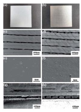
Fig. 4 Pictures and SEM images of the ABS and ABS-Ni membranes (left column represents ABS membranes, right column represents ABS-Ni membranes).
