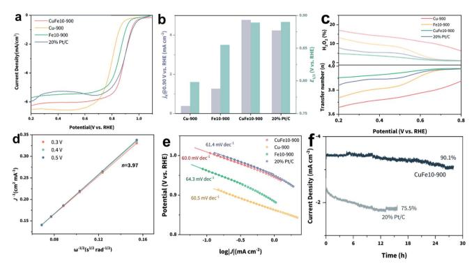
Fig. 3 (a) LSV curves, (b)  $j_k = 0.9 \text{ V}$  vs. RHE and  $E_{1/2}$  comparison, (c)  $H_2O_2$  selectivity and electron transfer number (n) of Cu-900, Fe10-900, CuFe10-900 and 20% Pt/C, (d) K-L plots of CuFe10-900, (e) Tafel plots of the four tested samples and (f) chronoamperometric tests of CuFe10-900 and Pt/C at 0.85 V vs. RHE.
