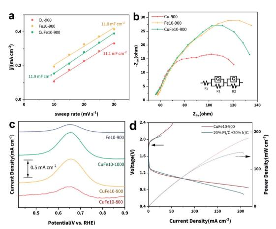
Fig. 4 (a)  $C_{\rm cl}$  fitting plots of Cu-900, Fe10-900 and CuFe10-900, (b) Nyquist plots of the three samples and equivalent circuit, (c) SWV curves of the four SACs and (d) charge–discharge and power density curves of CuFe10-900 and Pt/C for the Zn–air battery.
