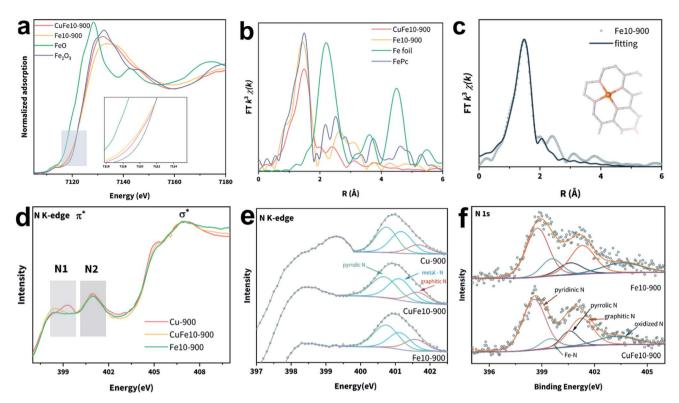
Fig. 2 (a) Fe K-edge XANES spectra, inset: magnified spectra, (b) FT-EXAFS spectra in the R space of CuFe10-900, Fe10-900 and standards (FeO and  $Fe_2O_3$ ), (c) first-shell fitting of the FT-EXAFS spectrum of CuFe10-900, (d) N K-edge XANES spectra and (e) magnified and deconvoluted N1 + N2 regions of the three SACs, and (f) deconvoluted N 1s XPS spectra of CuFe10-900 and Fe10-900
