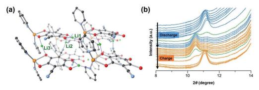
Fig. 5 (a) Computational simulation of lithiated CP  $[CuL(Py)_2Li_3]_n$  showing the DFT optimized structure. Colours of atoms: orange: Cu(i); grey: C; red: O; cyan: N; green: Li; H is omitted for clarity. (b) In situ synchrotron PXRD patterns of CP electrode collected during the first dischargecharge cycle at current density of 120 mA g<sup>-1</sup> at a voltage between 1.5 V and 4.0 V.
