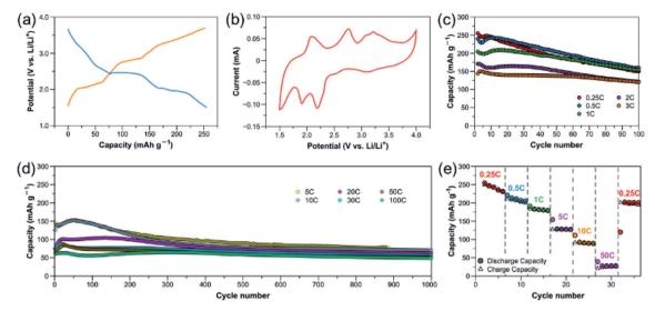
Fig. 2 Electrochemical properties of  $[CuL(Py)_2]_n$  cathode: (a) discharge–charge profile at 0.25C ( $\sim$ 65 mA g<sup>-1</sup>). (b) CV plot with a scan rate of 0.5 mV s<sup>-1</sup>. (c) Capacity retention at rates of 0.25C to 3C ( $\sim$ 785 mA g<sup>-1</sup>). (d) Capacity retention at rates of 5C ( $\sim$ 1308 mA g<sup>-1</sup>) to 100C ( $\sim$ 26 162 mA g<sup>-1</sup>). (e) Rate capability at various current densities.
