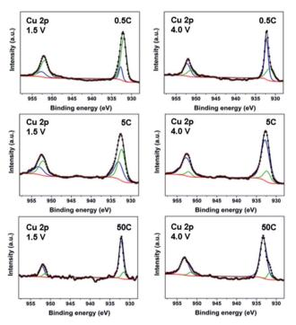
Fig. 3 Deconvolution of Cu  $2p_{3/2}$  and  $2p_{1/2}$  XPS spectra of  $[CuL(Py)_2]_n$  electrodes at various rates. 0.5C (top), 5C (middle) and 50C (bottom) at end of discharge (1.5 V, left) and end of charge (4.0 V, right) (green: Cu(0); blue: Cu(1)).
