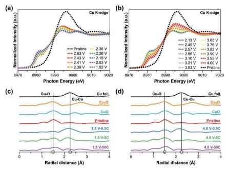
Fig. 4 XAS of  $[CuL(Py)_2]_n$  electrodes: (a) and (b) in situ Cu K-edge XANES patterns during discharge and charge at 20 mA  $g^{-1}$  ( $\sim 0.08C$ ), respectively. (c) and (d) Ex situ Cu K-edge EXAFS patterns at three different rates (0.5C, 5C and 50C) at end of discharge (1.5 V) and end of charge (4.0 V), respectively (with Cu foil, Cu<sub>2</sub>O and CuO as references).
