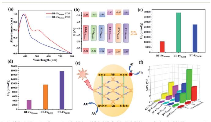
Fig. 8 (a) UV-vis diffuse absorption spectra of the BT-Py and BT-Cz COFs. (b) Calculated VB/CB energy levels of the COFs. Time course of the produced  $H_2$  of the (c) BT-Py<sub>Solvent</sub> COFs and (d) BT-Cz<sub>Solvent</sub> COFs for 4 h under irradiation with visible light ( $\lambda$  = 380–780 nm). (e) Schematic diagram of the photocatalytic  $H_2$  reduction over the COFs under visible light irradiation. (f) Wavelength dependence of AQY on the  $H_2$  evolution of the COFs.
