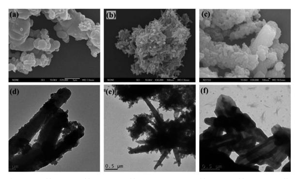
Fig. 3 FE-SEM images of (a) BT-Py<sub>Dioxane</sub>, (b) BT-Py<sub>BuOH</sub>, and (c) BT-Py<sub>EtOH</sub>. TEM images of (d) BT-Py<sub>Dioxane</sub>, (e) BT-Py<sub>BuOH</sub>, and (f) BT-Py<sub>EtOH</sub>.
