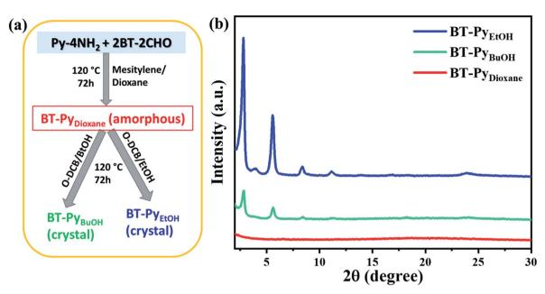
Fig. 7 (a) Schematic synthesis and (b) experimentally observed PXRD patterns of transforming amorphous material BT-Py<sub>Dioxane</sub> COF into crystalline BT-Py<sub>BuOH</sub> COF and BT-Py<sub>EtOH</sub> COF.
