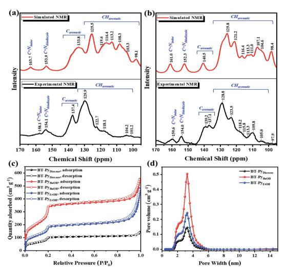
Fig. 2 Simulated and experimental 13C-NMR spectra of the (a) BT-Py<sub>Solvent</sub> COFs and (b) BT-Cz<sub>Solvent</sub> COFs. (c) N<sub>2</sub> adsorption (solid symbols) and desorption (open symbols) isotherms of the BT-Py<sub>Solvent</sub> COFs at 77 K. (d) The pore-size distribution of the BT-Py<sub>Solvent</sub> COFs.
