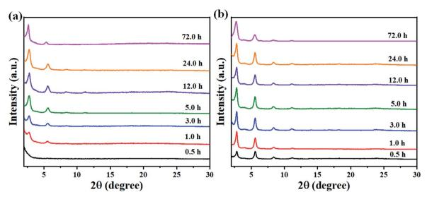
Fig. 6 Experimentally observed PXRD patterns of (a) BT-Py<sub>BuOH</sub> COF and (b) BT-Cz<sub>EtOH</sub> COF at different reaction times.
