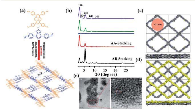
Fig. 1 (a) The synthesis of BT-Py<sub>Solvent</sub> COF; (b) experimental PXRD patterns of BT-Py<sub>Solvent</sub> (purple), Pawley refinement (green), their difference (blue), simulated profiles using AA-stacking (red), and AB-stacking (black) modes; unit cells of the (c) AA-stacking and (d) AB-stacking models; (e) high resolution TEM image of BT-Py COF.
