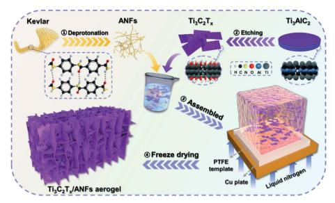
Scheme 1 Schematic illustration of the preparation of an anisotropic Ti<sub>3</sub>C<sub>2</sub>T<sub>x</sub>/ANF aerogel
