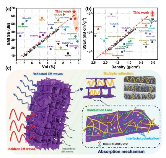
Fig. 6 (a) EMI SE versus  $Ti_3C_2T_x$  content (vol%) and (b) SSE/t versus density of the anisotropic  $Ti_3C_2T_x/ANF$  aerogels compared with previous reports. (c) Electromagnetic shielding mechanism of the anisotropic Ti<sub>3</sub>C<sub>2</sub>T<sub>x</sub>/ANF aerogel.
