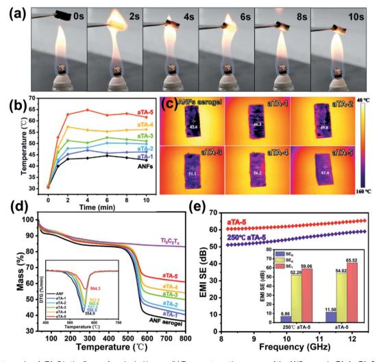
Fig. 7 (a) Photographs of aTA-5 in the flame of an alcohol burner. (b) Temperature–time curves of the ANF aerogel, aTA-1, aTA-2, aTA-3, aTA-4, aTA-5 and  $Ti_3C_2T_x$ . (c) A series of infrared thermal imager photos of the  $Ti_3C_2T_x$ /ANF composite aerogels placed on a heating table at 150 °C. (d) TGA and DTA curves of a series of MXene/ANF composite aerogels. (e) EMI SE, SE<sub>T</sub>, SE<sub>A</sub> and SE<sub>R</sub> of aTA-5 before and after treatment at 250 °C for 2 hours.
