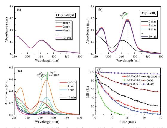
Fig. 12 (a) Reaction of Cr(vi) with only MoCoOS-2, (b) reaction of Cr(vi) with only NaBH<sub>4</sub>, (c) reduction of Cr(vi) with MoCoOS-2 and NaBH<sub>4</sub>, (d) reduction of Cr(vI) with Mo(S,O), Co(O,S), and MoCoOS catalysts in the presence of NaBH<sub>4</sub>.
