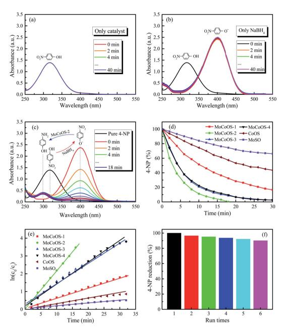
Fig. 8 (a) Reaction of 4-NP with MoCoOS-2. (b) Reaction of 4-NP with NaBH $_4$ . (c) Reduction of 4-NP with MoCoOS-2 and NaBH $_4$ . (d) Reduction of 4-NP with Mo(S,O), Co(O,S), and MoCoOS catalysts in the presence of NaBH $_4$ . (e) The first order reaction rate curves of 4-NP. (f) Catalytic reduction efficiency after cycles of reactions.
