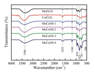
Fig. 3 FTIR spectra of Mo(S,O), Co(O,S), and MoCoOS prepared with different amounts of CoCl $_2\cdot$ 6H $_2$ O.
