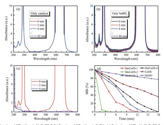
Fig. 10 (a) Reaction of MB with only MoCoOS-2 and NaBH<sub>4</sub>. (d) Reduction of MB with MoCoOS-2 and NaBH<sub>4</sub>. (d) Reduction of MB with Mo(S,O), Co(O,S), and MoCoOS catalysts in the presence of NaBH<sub>4</sub>.
