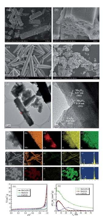
Fig. 4 (a and b) SEM images of MoCoOS-2. SEM images of (c) Mo(S,O) and (d) Co(O,S). (e) TEM and (f) HR-TEM images of MoCoOS-2. (g-k) EDX element distribution mapping images of Mo, Co, O, and S for MoCoOS-2. (1-p) EDX element distribution mapping images of Mo, O, and S for Mo(S,O). (q-u) EDX element distribution mapping images of Co, O, and S for Co(O,S). (v) Nitrogen adsorption-desorption isotherm and (w) the pore size distribution curve of the catalysts.
