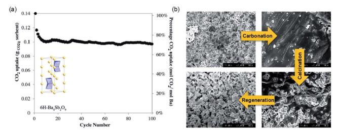
Fig. 15 (a) CO<sub>2</sub> uptake by 6H perovskite Ba<sub>4</sub>Sb<sub>2</sub>O<sub>9</sub> over 100 carbonation-calcination cycles in at TGA. (b) Surface morphology Ba<sub>4</sub>Sb<sub>2</sub>O<sub>9</sub> as it evolves over carbonation-calcination cycles. Reprinted with permission<sup>155</sup> copyright 2021 American Chemical Society.
