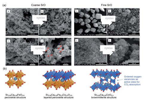
Fig. 14 (a) SEM images of coarse and fine SrO particles before (A & C) and after five cycles (B & D) of carbonation—calcination at 1100 °C (b)  $Sr_{0.95}Ca_{0.05}Fe_{0.5}Co_{0.5}O_{3-\delta}$  perovskite with a layered structure and its phase segregation to a Fe-rich and a Co-rich phase. The undercoordinated Co sites are considered to be the preferential sites for CO<sub>2</sub> absorption. Reprinted with permission<sup>144</sup> copyright 2021 American Chemical Society.
