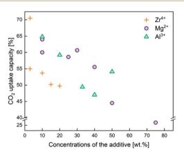
Fig. 4 CO<sub>2</sub> capture capacity of CaO based sorbents stabilised by the three different typical sintering-resistant, oxidic additives containing Zr<sup>4+</sup>, Al<sup>3+</sup>, and Mg<sup>2+</sup>. The effect of these additives on the cyclic stability of CaO sorbents is summarised in Table 2.
