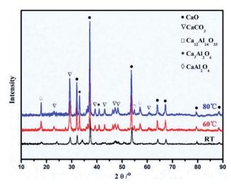
Fig. 6 XRD patterns of the Ca–Al mixed oxides ( $Ca^{2+}/Al^{3+} = 3$ ) svnthesised at room temperature (RT), 60 °C and 80 °C. Reprinted with permission66 copyright 2021 Elsevier.
