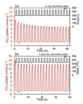
Fig. 8  $CO_2$  capture capacity of promoted MgO by alkali metal nitrates ((Li-Na-K)NO<sub>3</sub>) and nitrate/nitrite (LiNO<sub>3</sub>-(Na-K)NO<sub>2</sub>) salt. Reprinted with permission<sup>86</sup> copyright 2021 American Chemical Society.
