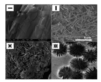
Fig. 10 SEM images of the structure of MgO sorbents: plate, <sup>96</sup> rod, <sup>97</sup> and fuzz-like structure of MgO sorbents<sup>95</sup> and TEM image of the flower-like plate, <sup>98</sup> Reprinted with permission copyright 2021 American Chemical Society. <sup>96</sup> Reprinted with permission copyright 2021 Royal Society of Chemistry, <sup>95</sup> Reprinted with permission copyright 2021 John Wiley and Son, Inc. <sup>97,98</sup>
