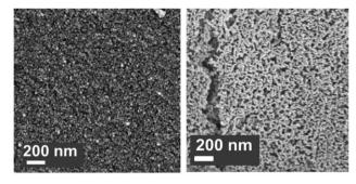
Fig. 3 Scanning electron micrograph of CaO stabilised with both MgO and Al<sub>2</sub>O<sub>3</sub> (left) as-synthesised and (right) after 23 cycles of carbonation/calcination.56
