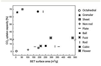
Fig. 9 CO<sub>2</sub> uptake capacity and BET surface area according to the various structure of MgO sorbents. The data points entries are obtained from ref. 84, 92, 95, 96, 98 and 99.
