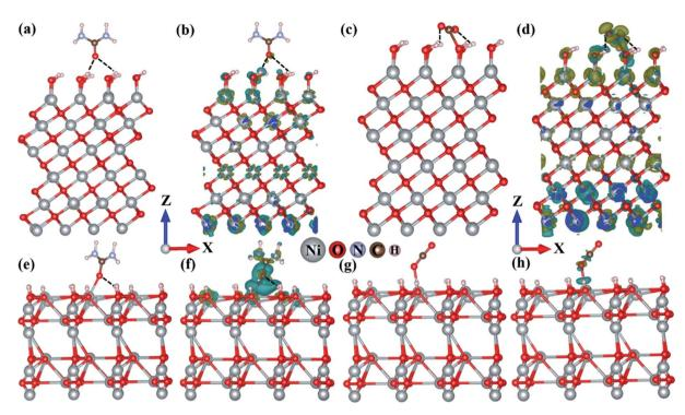
Fig. 9 Optimized structures and corresponding charge density difference (CDD) plots: (a and b) urea adsorbed, (c and d) CO2 adsorbed Niterminated hydroxylated NiO (111) surface, (e and f) urea adsorbed, (g and h) CO<sub>2</sub> adsorbed hydroxylated Ni<sub>2</sub>O<sub>3</sub> (002) surface. Isodensity value at surfaces is  $\pm 0.004$  e a.u.<sup>-3</sup> (positive: cyan and negative: olive).
