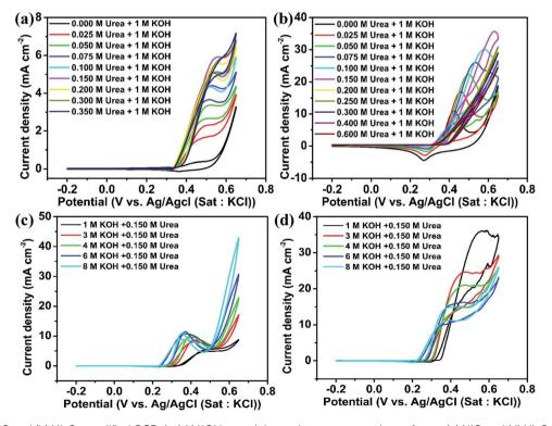
Fig. 5 CV of (a) NiO and (b) Ni<sub>2</sub>O<sub>3</sub> modified GCEs in 1 M KOH containing various concentrations of urea: (c) NiO and (d) Ni<sub>2</sub>O<sub>3</sub> in different molar concentrations of KOH with a fixed urea concentration of 0.150 M at a scan rate of 10 mV s<sup>-1</sup>.
