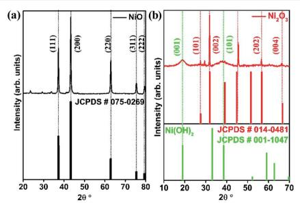
Fig. 1 XRD pattern of (a) NiO and (b) Ni<sub>2</sub>O<sub>3</sub>.
