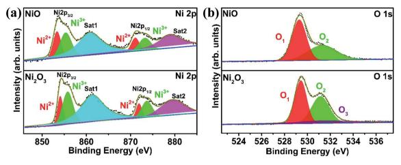
Fig. 3 High-resolution XPS of NiO and Ni<sub>2</sub>O<sub>3</sub>: (a) Ni 2p spectra and (b) O 1s spectra.
