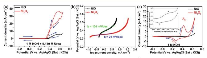
Fig. 4 (a) CV of NiO and Ni<sub>2</sub>O<sub>3</sub> in 1 M KOH containing 0.150 M urea at a scan rate of 10 mV s<sup>-1</sup>, (b) Tafel slope of NiO and Ni<sub>2</sub>O<sub>3</sub> in 1 M KOH + 0.150 M urea, and (c) CV of NiO and Ni<sub>2</sub>O<sub>3</sub> in 1 M KOH at a scan rate of 10 mV s<sup>-1</sup> along with the magnified view of the redox region of NiO in the inset.
