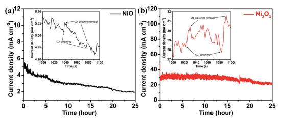
Fig. 8 i-t curves monitored for 25 hours for (a) NiO in 6 M KOH + 0.150 M urea at 0.40 V vs. Ag/AgCl<sub>(sat.KCl)</sub> and (b) the Ni<sub>2</sub>O<sub>3</sub> catalyst in 1 M KOH + 0.150 M urea at 0.58 V vs. Ag/AgCl<sub>(sat.KCl)</sub>; insets show the enlarged view of current density fluctuations.
