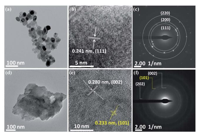
Fig. 2 TEM images of NiO (a–c) and Ni<sub>2</sub>O<sub>3</sub> (d–f). (a) NiO crystallites, (b) HRTEM of NiO, (c) SAED pattern of NiO and (d) Ni<sub>2</sub>O<sub>3</sub> sheets, (e) HRTEM of Ni<sub>2</sub>O<sub>3</sub> sheets and (f) SAED pattern of Ni<sub>2</sub>O<sub>3</sub> sheets (HRTEM and SAED of Ni(OH)<sub>2</sub> are highlighted in yellow color).
