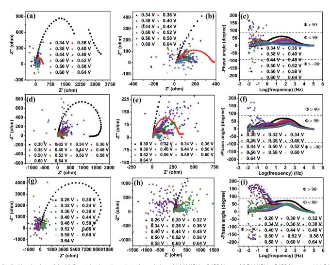
Fig. 7 Nyquist plots of the Ni<sub>2</sub>O<sub>3</sub> catalyst in various electrolyte solutions: (a) 1 M KOH + 0.150 M urea, (d) 3 M KOH + 0.150 M urea and (g) 6 M KOH + 0.150 M urea. (b), (e) and (h) Enlarged views of the semicircle in the high-frequency region of (a), (d) and (g). Corresponding Bode plots in (c) 1 M KOH + 0.150 M urea, (f) 3 M KOH + 0.150 M urea and (i) 6 M KOH + 0.150 M urea.
