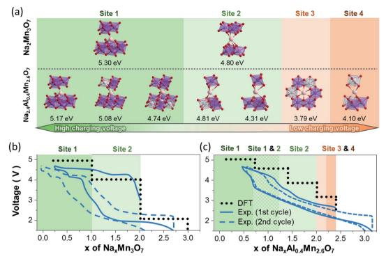
Fig. 4 (a) Local bonding environment of Na sites and their predicted Na vacancy formation energies in Na<sub>x</sub>Mn<sub>3</sub>O<sub>7</sub> and Na<sub>x</sub>Al<sub>0.4</sub>Mn<sub>2.6</sub>O<sub>7</sub>. Theoretical and experimental voltage profiles of (b)  $Na_xMn_3O_7$  and (c)  $Na_xAl_{0.4}Mn_{2.6}O_7$ . Electrochemically active  $Na_x$  sites for each  $Na_x$  content range are highlighted in differing colours.
