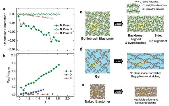
Fig. 7 (a) Orientation parameter (f) measured by SAXS for peaks L and H of **B** and **N** and (b) the deviations from the nH model based on the uniaxial stress–strain data for the three networks. The first data point in each data series in Panel b has been omitted due to large error. (c–e) Schematic illustration of the structural changes in the three networks during uniaxial deformation.
