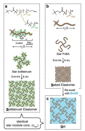
Fig. 1 Preparation scheme for the three model networks used in this study. (a) Bottlebrush elastomer  ${f B}$ . (b) "Naked" elastomer  ${f N}$ . (c) Gel  ${f G}$ . All three networks had almost identical polymerization degrees between cross-links  $(n_{\rm x})$  by design.  ${\bf G}$  was prepared so that the number density of the star polymer module ( $c_{\text{star}}$ ) was identical to that of **B**. The networks are illustrated in 2D for the sake of simplicity.
