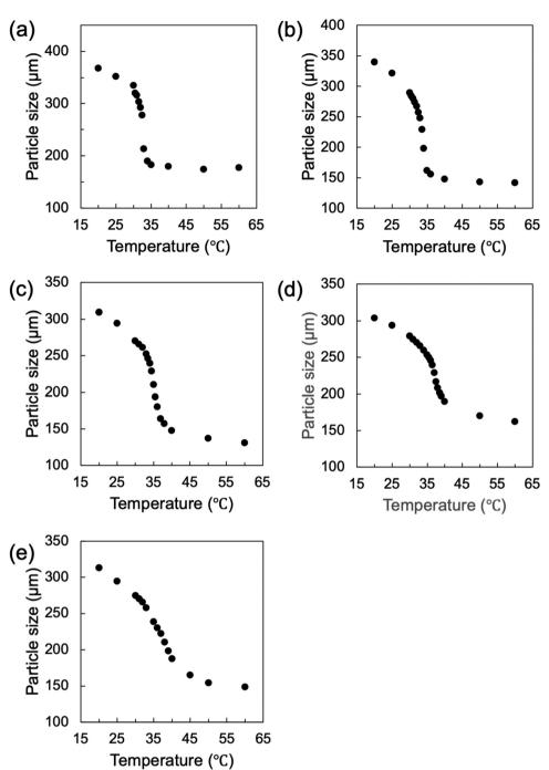
Fig. 6 Diameter of the spherical gels (a) PNIPA gel, (b) PNIPA<sub>0.9</sub>-b-PDMA<sub>0.1</sub> gel, (c) PNIPA<sub>0.8</sub>-b-PDMA<sub>0.2</sub> gel, (d) PNIPA<sub>0.7</sub>-b-PDMA<sub>0.3</sub> gel and (e) PNIPA<sub>0.8</sub>-r-PDMA<sub>0.2</sub> gel at equilibrium at certain temperature for each of them. The diameters are measured through an inverted optical microscope.
