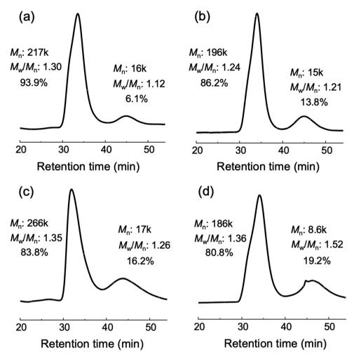
Fig. 4 SEC curve obtained after methanolysis decomposition of (a) PNIPA gel, (b)PNIPA $_{0.9}$ -b-PDMA $_{0.1}$  gel, (c) PNIPA $_{0.8}$ -b-PDMA $_{0.2}$  gel and (d) PNIPA $_{0.7}$ -b-PDMA $_{0.3}$  gel.
