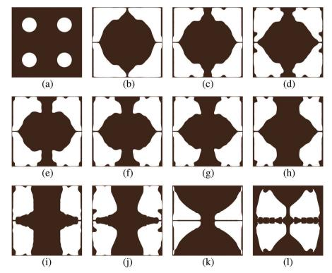
Fig. 6 (a) Initial design with four holes in the whole design domain; (b)–(l) Final designs with different weights  $\omega=0,\,0.1,\ldots,\,1.$
