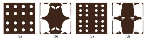
Fig. 8 (a and c) Initial designs with 16 holes and 24 holes, and (b and d) the corresponding final results obtained with  $\omega = 0.5$ .
