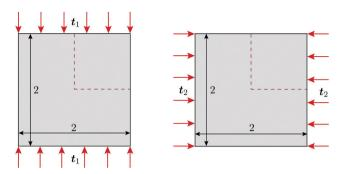
A domain with dimension 2  $\times$  2 under compression, where  $\mathbf{t}_1$  and t<sub>2</sub> are prescribed on the vertical and horizontal directions, respectively. Under the finite element analysis, a quarter of domain (marked with red dashed segments) is considered.
