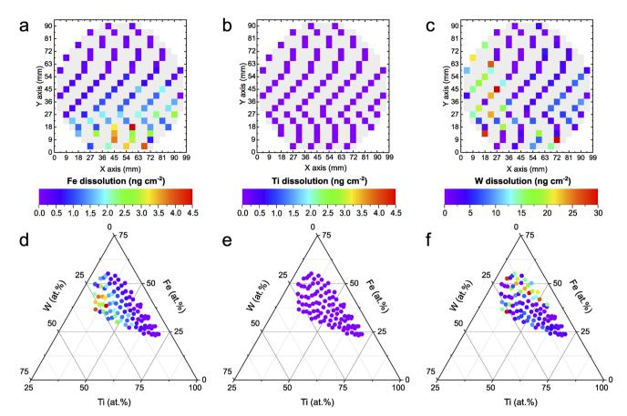
Fig. 2 Element-specific dissolution of Fe-Ti-W-O material library at 1.7 V<sub>RHE</sub>. (a-c) Dissolved amounts of Fe (a), Ti (b), and W (c) mapped onto a schematic representation of the wafer. (d-f) Dissolved amounts of Fe (d), Ti (e), and W (f) mapped onto a ternary diagram. The HT measurements were conducted in  $0.05 \,\mathrm{M}$  NaNO<sub>3</sub> (pH 5.7) under 1 Sun Am 1.5G illumination. Note that the color scale for W differs from Fe and Ti.
