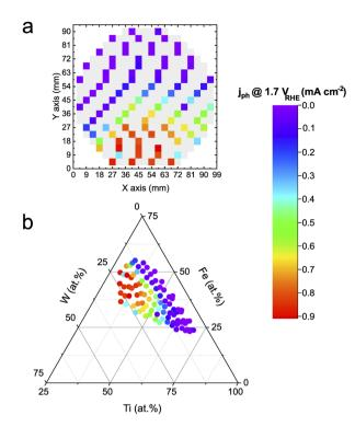
Fig. 1 Photocurrent densities of Fe–Ti–W–O material library at 1.7  $V_{RHE}$ . (a) Photocurrent density mapped onto a schematic representation of the wafer. (b) Photocurrent density mapped onto a ternary composition diagram of the metal constituents. The HT measurements were conducted in 0.05 M NaNO $_3$  (pH 5.7) under 1 Sun Am 1.5G illumination.
