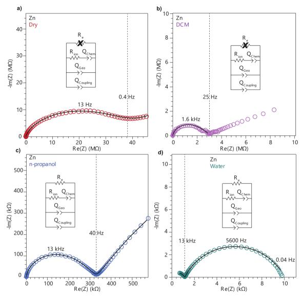
Fig. 4 Nyquist plots of  $TMA_2ZnGe_4S_{10}$  pressed-pellets when dry (a) and after addition of DCM (b), n-propanol (c), and deionized water (d). Black traces represent fits to the equivalent circuit diagrams shown in the figure. Crossed-out circuit elements denote elements that are too large to adequately fit to the impedance response.
