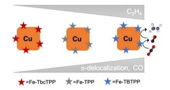
Fig. 8 Schematic representation of the proposed mechanism for  $C_2H_4$  promotion in  $Cu_{cub}/Fe-Por$  tandem catalysts. The C–C coupling enhancement and  $C_2H_4$  promotion correlate with the Fe-Por selectivity and conversion rate for CO.
