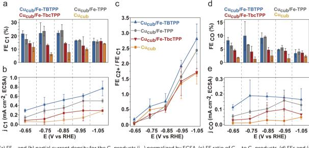
Fig. 5 (a) FE<sub>C</sub>, and (b) partial current density for the  $C_1$  products  $(j_{C_1})$  normalized by ECSA, (c) FE ratio of  $C_{2+}$  to  $C_1$  products, (d) FEs and (e) partial current density for CO  $(j_{CO})$  normalized by ECSA of  $Cu_{cub}/Fe-TBTPP$ ,  $Cu_{cub}/Fe-TPP$ ,  $Cu_{cub}/Fe-TDETPP$  and  $Cu_{cub}$  at different potentials. The reported values are an average of three independent experiments with error bars indicating the standard deviations.
