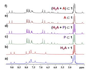
Fig. 6 Partial  $^1H$  NMR stack plot of (a) 1, (b)  $(H_2A+1)$   $(H_2A=9.10-dihydroanthracene)$ , (c)  $P \subset 1$  (P: phenanthrene), (d)  $(H_2A+P) \subset 1$ , (e)  $A \subset 1$  (A: anthracene) and (f)  $(H_2A+A) \subset 1$  in  $D_2O$  showing the selective encapsulation of A and P.
