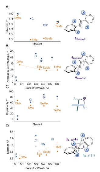
Fig. 5 Geometric parameters from single-crystal data for (E)- $X_4$  (A) C-N=N-C dihedral, (B) average N=N-C-C dihedral, (C) coplanarity of rings, (D) distances between diazo lone pair and X-atom (formation of intramolecular 5 ( $\spadesuit$ ) and 4 ( $\square$ ) membered rings).
