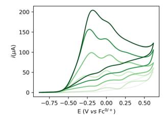
Fig. 3 CV of 5 mM NaOEt (grey), 5 mM of 1 + 1 M EtOH with varying concentrations of base (5, 10, 15, and 20 mM NaOEt, light to dark green) in 2:1 THF/DFB + 0.2 M NaPF<sub>6</sub>. Scan rate 0.1 V s<sup>-1</sup>, electrode: 3 mm diameter GC electrode.
