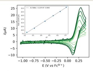
Fig. 1 Scan rate dependence of a 1 mM solution of 1 in in 2:1 THF/ DFB + 0.2 M NaPF6 (from light to dark green: 0.05, 0.1, 0.2, 0.3, 0.4 and 0.5 V s<sup>-1</sup>, 3 mm GC electrode). Inset: evolution of the peak current as a function of the square root of the scan rate.
