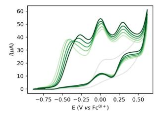
Fig. 2 CVs of 10 mM NaOEt (grey) and of 5 mM 1 + 5 mM NaOEt with increasing concentrations of EtOH (from light to dark green: 200, 400, 600, 800 and 1000 mM) in 2:1 THF/DFB + 0.2 M NaPF<sub>6</sub>. Scan rate 0.1 V s<sup>-1</sup>, electrode: 3 mm diameter GC electrode.
