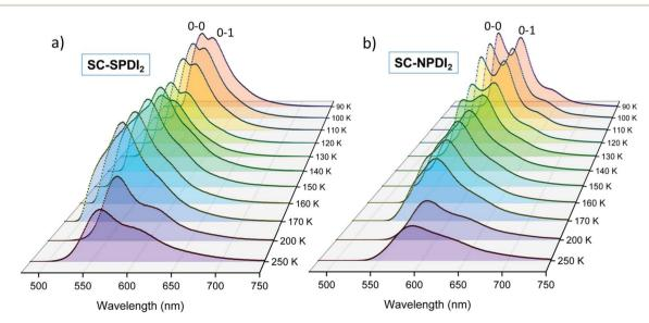
Fig. 3 The temperature-dependent photoluminescence spectra of (a) SC-SPDI<sub>2</sub> and (b) SC-NPDI<sub>2</sub> in toluene.
