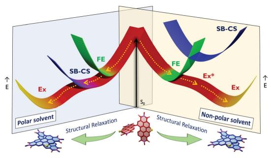
Fig. 6 The potential energy diagram summarizes the excited-state dynamics of SC-SPDI2 and SC-NPDI2 undergoing structural relaxation in polar solvents (ACE and ACN) and non-polar solvent (TOL), where FE is the Frenkel exciton, Ex\* is the unrelaxed excimer state, Ex is the stable excimer state and SB-CS is the symmetry-breaking charge-separated state. The x-axis represents the reaction coordinate and E on the y-axis indicates the potential energy.
