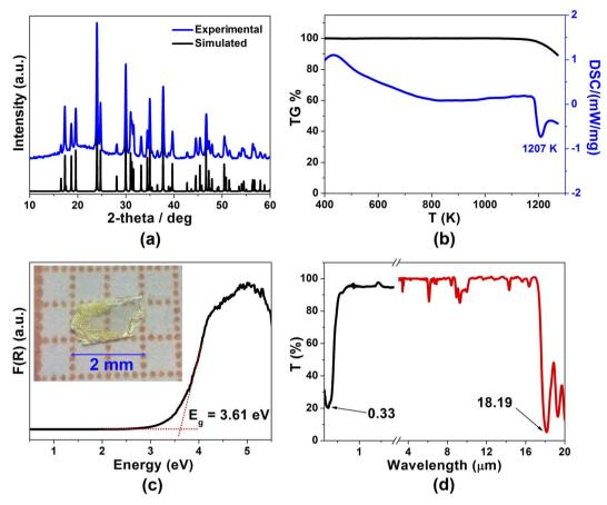
Fig. 1 Experimental characterization results of  $SrCdSiS_4$ : (a) experimental (blue) and simulated (black) powder XRD curves; (b) TG and DSC diagrams; (c) solid-state UV-vis-NIR diffuse reflectance spectrum (inset: photograph of a polished crystal); (d) optical transmittance spectra from UV-vis to IR region.
