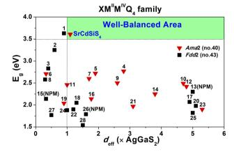
Fig. 4 Comparison of  $d_{eff}$  and  $E_q$  of the  $XM^{II}M^{IV}Q_4$  system (X = Eu, Sr, Ba;  $M^{II} = Mn$ , Zn, Cd, and Hg;  $M^{IV} = group-14$  elements; and Q = group-14chalcogen) and the green shaded region represents the well-balanced  $(E_q > 3.5 \text{ eV} \text{ and } d_{\text{eff}} > 1.0 \times \text{AgGaS}_2)$  area for IR-NLO materials. Details are listed in Table S4.†
