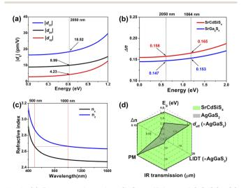
Fig. 6 (a) Frequency-dependent SHG coefficients of SrCdSiS<sub>4</sub>; (b) curves of the calculated  $\Delta n$  as a function of energy (eV) for SrGa<sub>2</sub>S<sub>4</sub> and SrCdSiS<sub>4</sub>; (c) calculated refractive index dispersion curves with the shortest PM cut-off edge at 500 nm; (d) radar chart with six directions (representing  $E_{\rm g}$ ,  $d_{\rm eff}$ , LIDT, IR transmission, PM,  $\Delta n$ ) to characterize comprehensive IR-NLO performance of SrCdSiS<sub>4</sub>.
