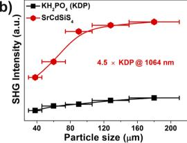
Fig. 3 Phase-matching curves for SrCdSiS<sub>4</sub> and inserted values are the SHG intensities in the particle size range of  $150-210 \mu m$ : (a) AgGaS<sub>2</sub> as the benchmark under 2050 nm radiation; (b) KDP as the reference under 1064 nm radiation. The solid curves are drawn as a guide to the eye.
