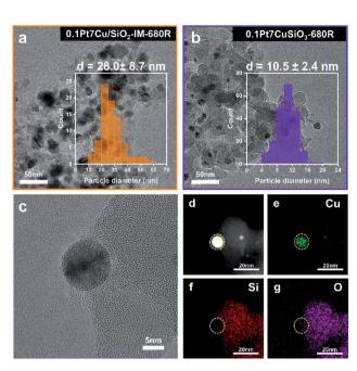
Fig. 2 Typical TEM images and particle size distributions of (a)  $0.1 \text{Pt7Cu/SiO}_2\text{-IM}-680\text{R}$  and (b)  $0.1 \text{Pt7CuSiO}_3-680\text{R}$ . (c) Representative TEM images of  $0.1 \text{Pt7CuSiO}_3-680\text{R}$ . (d) Corresponding HAADF-STEM images including elemental maps of (e) Cu, (f) Si, and (g) O of  $0.1 \text{Pt7CuSiO}_3-680\text{R}$  acquired by EDS. PtCu SAA is highlighted by the yellow dotted circle.
