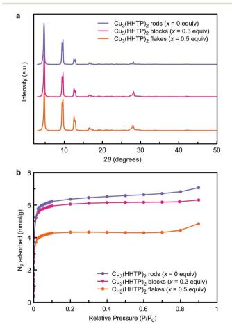
Fig. 4 (a) Powder X-ray diffraction patterns and (b) surface areas of  $\text{Cu}_3(\text{HHTP})_2$  synthesized with 0, 0.3, and 0.5 equiv. of 2,5-dichloro-1,4-benzoquinone pre-oxidant.
