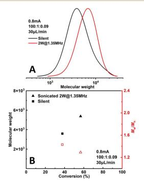
Fig. 6 Comparison of polymerizations of methyl acrylate under silent and sonicated conditions.
