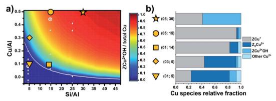
Fig. 4 (a) Predicted Cu site compositional phase diagram *versus* Si/Al and Cu/Al ratios. Color scale indicates predicted fraction of ZCu<sup>2+</sup>OH. Adapted with permission from ref. 85. Copyright 2016 American Chemical Society. (b) Relative fractions of Cu species; the label "other Cu<sup>2+</sup>" refers to very minor contributions from residual, partially hydrated Cu<sup>2+</sup> species. Unpublished figure reporting data from ref. 86.
