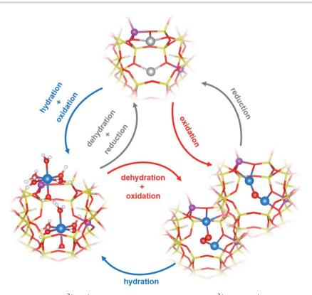
Fig. 2 Examples of redox cycles involving  $Cu^{2+}/Cu^+$  ions in DMTM. Colour code: blue,  $Cu^{2+}$ ; gray,  $Cu^+$ ; yellow, Si; magenta, Al; red, O; white, H. Unpublished figure, structural models from ref. 81.
