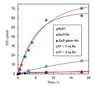
Fig. 5 CO formation with time under irradiation from LED lamps at 560 nm with a merry-go-round apparatus for CO<sub>2</sub>-saturated DMA-TEOA (5:1 v/v, total 1.0 mL) solutions containing BIH (0.1 M) in the presence of ReD' (0.025 mM), ReD'Re (0.025 mM), ZnP-phen=Re (0.050 mM), and a mixed system of D' (0.025 mM) and fac- $Re(bpy)(CO)_3Br (Re: 0.025 mM or 0.05 mM).$
