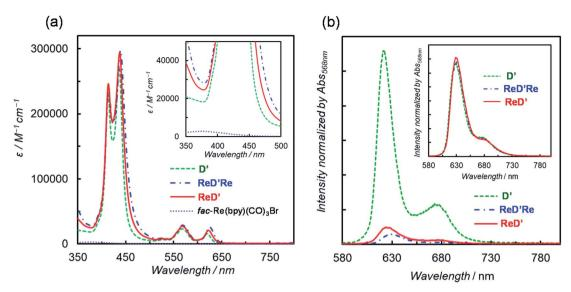
Fig. 3 (a) UV-vis absorption spectra of D', ReD', ReD', and fac-Re(bpy)(CO)<sub>3</sub>Br in DMA. The inset presents the magnification of the near-UV region. (b) Fluorescence spectra of D', ReD'Re, and ReD' in DMA at 298 K. The inset shows the spectra in toluene. The fluorescence spectra were normalized with the absorbance at the excitation wavelength ( $\lambda_{ex} = 568$  nm).
