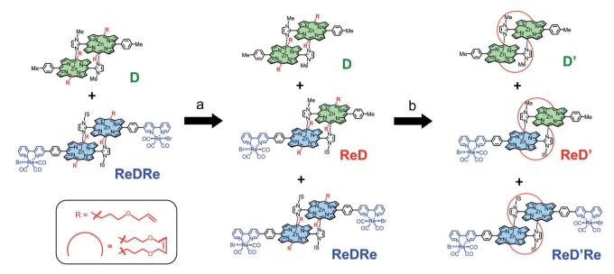
Scheme 3 Synthesis of the heterodimer, ReD'. Reagents and conditions: (a) (i) mixing in pyridine at rt, (ii) evaporating the solvent *in vacuo*; (b) Grubbs catalyst (0.5 equiv.), CHCl<sub>3</sub>, and rt.
