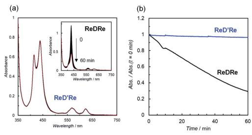
Fig. 10 (a) UV-vis absorption spectral change of a CO<sub>2</sub>-saturated DMSO-TEOA ( $5:1\,\text{v/v}$ ) solution containing BIH (0.01 M) and ReD'Re ( $2.5\,\mu\text{M}$ ) during irradiation at 560 nm (Xe lamp,  $3.5\times10^{-8}$  einstein s<sup>-1</sup>) and 25 °C. Inset shows change using ReDRe instead of ReD'Re. Red dotted lines show the spectra after the irradiation for 60 min. (b) Relative absorbance with time at 430 nm of the reaction solutions during the irradiation.
