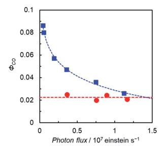
Fig. 7  $\Phi_{CO}$  as a function of light irradiation intensity (Xe lamp,  $\lambda_{ex}=560$  nm) for ReD' (0.1 mM) in DMA-TEOA (5 : 1 v/v) solutions containing BIH (0.1 M) (red circles) and ZnP-phen=Re (0.3 mM) in DMA solutions containing BIH (0.05 M) and PhOH (0.1 M) (blue squares).
