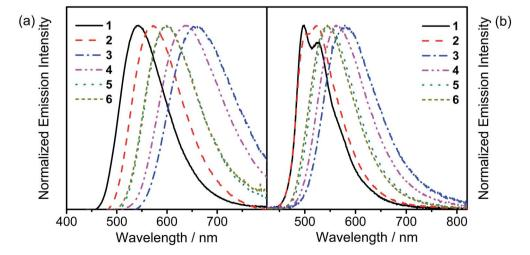
Fig. 1 (a) Normalized PL spectra of 1-6 in degassed toluene at 298 K. (b) Normalized PL spectra of thin films of 20 wt% 1-6 doped in MCP at 298 К.
