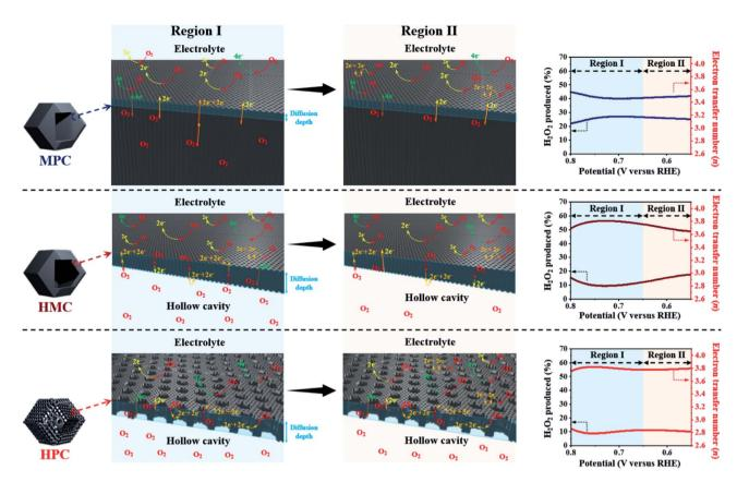
Fig. 4 Graphical description of proposed effect of different nanoarchitectures (MPC, HMC and HPC) on overall electron transfer number calculated from RRDE method ( $4e^-$ ,  $2e^- + 2e^-$  and  $2e^-$  indicate four electron, double two electron and single two electron transfer pathways, respectively).
